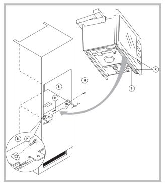
Fix the fastening bar such that the two lips stick out over the edge of the bottom of the recess and rest against it at the front.
